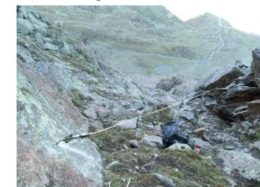
Steel tape extensometer measurement at a scar of a deep seated sagging of mountain slope.
