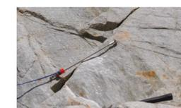
electrical crackmeter at al large joint directly above the contemporary glacier margin.
