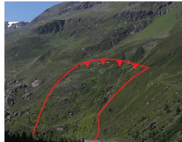
Deeper seated large landslide (above) in the 1850 moraine deposits of the gepatsch glacier and the associated section of the Arc-Gis based geotechnical map.
