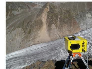
The results of repeated high-resolution airborne laser scanning (ALS) will contribute to a complete area-wide detection of surface changes and facilitates geomorphic mapping. Detailed periodical terrestrial laser scanning (TLS) of steep rock walls and their scree cones will complete the data set. Spot tests with rock fall collector nets, constructed on elected scree cones, allow the verification of the TLS data.
