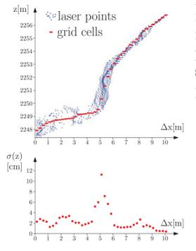
The least squares adjustment performed for the tilted plane interpolator allows the estimation of the **grid height precision  $\sigma(z)$** . As can be seen in Fig.6,  $\sigma(z)$  mainly depends of:
