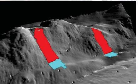
Calculation of the rockwall source area on a DEM1 (blue: rockfall collector nets)
