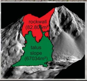
Example of the ,talus production ratio' (after COE & HARP 2007) on the base of a DEM5. The talus production ratio is the area ratio between talus slope and rock wall. It gives an impression of the rockfall susceptibility of different rock masses on a larger scale, as long as talus slopes under similar conditions (e.g. unconstrained deposition, similar talus production timeframe) are compared.
