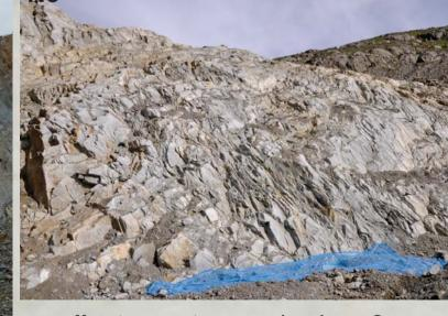
collector nets: mesh size: 2mm; net area: 80-230m², fixed by iron hooks at the base of the rockwall
