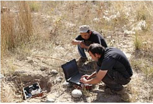
Project team member Florian Betz checking a soil humidity measuring instrument at the Naryn floodplains in the context of an earlier project. Soil humidity is one of the most important parameters for a natural development of floodplain vegetation. (Photo: Rauschenberger/upd)
